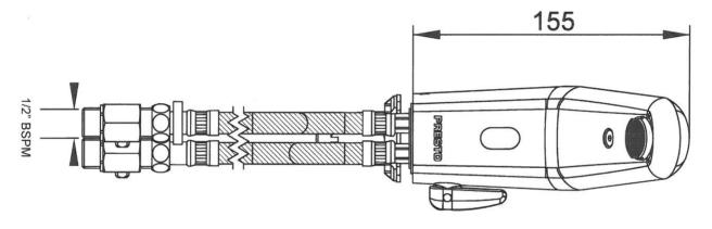
Presto Volta Sensor Mixer Tap (Battery) www.thornthwaite.com.au
