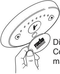
Disable the Control Panel with the magnetic key.
