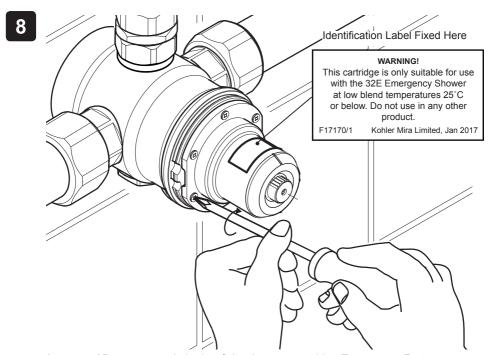
**Important!** Do not remove hub when fitting the spare cartridge. Temperature Factory preset must not be adjusted
