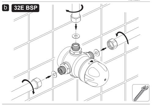
32E shown. The rest of the installation procedure is similar for all variants of the 32 valve.
