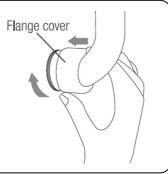
When marking out these grab rails, use centre base holes of flange protector.
