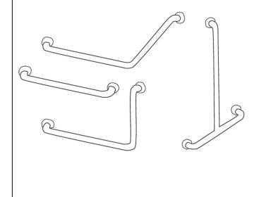
When marking out corner grab rails and corner of rail is left of the flange, mark base holes CORNER TO LEFT. If corner rail is right, mark base holes CORNER TO RIGHT
