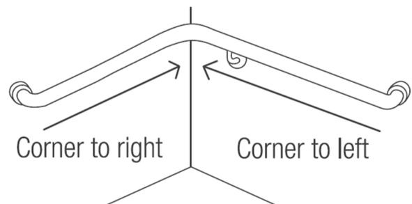
NOTE: Do not use FLANGE PROTECTOR INSTALLATION GUIDE for corner grab rails if screws have to be positioned vertically.
