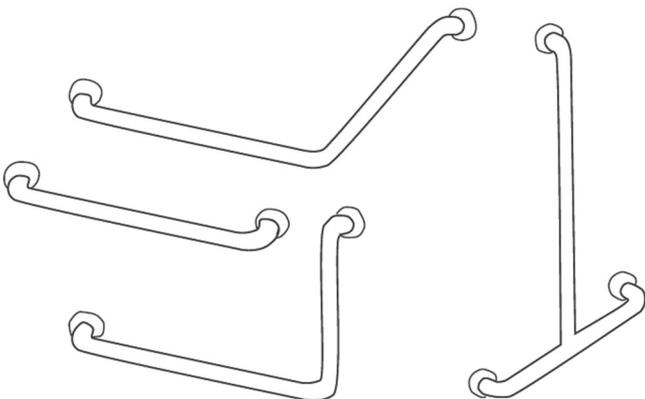
When marking out corner grab rails and corner of rail is left of the flange, mark base holes CORNER TO LEFT. If corner rail is right, mark base holes CORNER TO RIGHT
