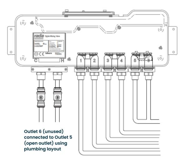
Do not install additional TMVs in the pipework that supplies water to or from Rada Outlook
