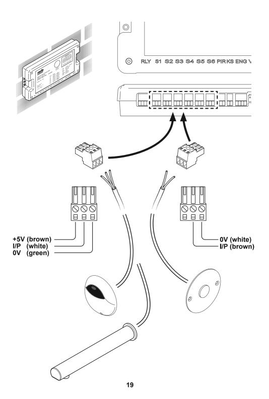
This product is compliant with all CE marking directives with sensor cables up to 6 meters in length. Should the cable be extended beyond this length, you must make sure the installation complies with all relevant directives and local regulations.
